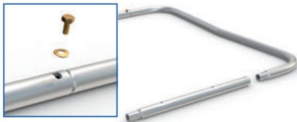
fig. 3: Assembly of the feet
